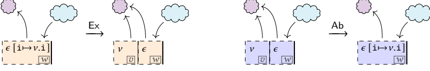
Fig. 11. Schematic depictions of the expel (left) and absorb (right) rewrite rules, that focus on the segment of the dovetailed messages together with all pointers into and out of them, within a particular memory snapshot. The circular cloud represents the subset of the memory that the messages in focus are pointing to, showing their views are the same. The elliptical cloud represents views—possibly including the initial and final view, as well as other messages—that point to each of the dovetailing messages. Thus, no view may point to v . A condition that is not depicted is that all the messages must appear in the same places in the chronicle. Left: The environment message v is “expelled” from the message \epsilon' , which becomes \epsilon . Right: The local message v is “absorbed” into the message \epsilon , which becomes \epsilon' .
